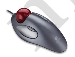
A **trackball** is a computer pointing device which can perform the same functions as a mouse. When a user moves the mouse, the ball rolls, causing the pointer on the screen to move. With a trackball, the user simply rolls the ball itself using her fingers or thumb, while the body of the device stays in place.
