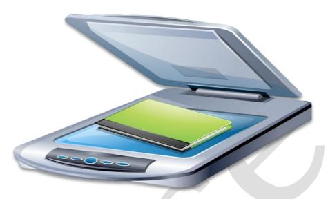
A **scanner** is a device that captures images from photographic prints, posters, magazine pages, and similar sources for computer editing and display. Scanners come in hand-held, feed-in, and flatbed types and for scanning black-and-white or color.
